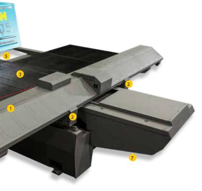
On the large standard brush tables, various workpieces can be nested on standard sheet sizes. The fast AC-servo driven X- and double Y-axes with resp. stroke of 2540 by 1580 mm (100" by 62") or 3000 by 1580 mm (120" by 62") and 3 hydraulic sheet clamps with minimal 'dead zone' 225 by 95 mm (8.85" by 3.74") ensure the highest accuracy on all workpieces.
