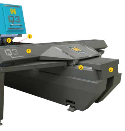
On the large standard brush tables, various workpieces can be nested on standard sheet sizes. The fast AC-servo driven X- and Y-axes with resp. stroke of 2032 by 1524 mm (80" by 60") on Q3 or 2540 by 1524 mm (100" by 60") on Q4 and 3 hydraulic sheet clamps with minimal 'dead zone' 225 by 95 mm (8.85" by 3.74") ensure the highest accuracy on all workpieces (optional CNC programmable).
