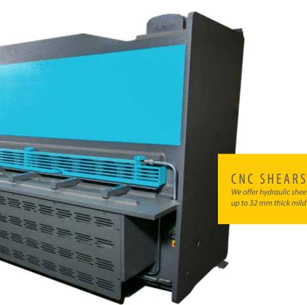
We offer hydraulic sheet metal guillotine shears that can cut up to 32 mm thick mild steel sheets, up to 6 m long.
