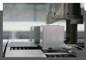
Exceptionally fast forming capabilities. With a bending height of 70mm (2.75") in a variety of angles and even on parts which are nested in other locations than 0° - 45° and 90° your punch press becomes a multifunctional part processing machine.
