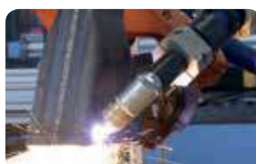
Fasenschneiden Bevel cutting
